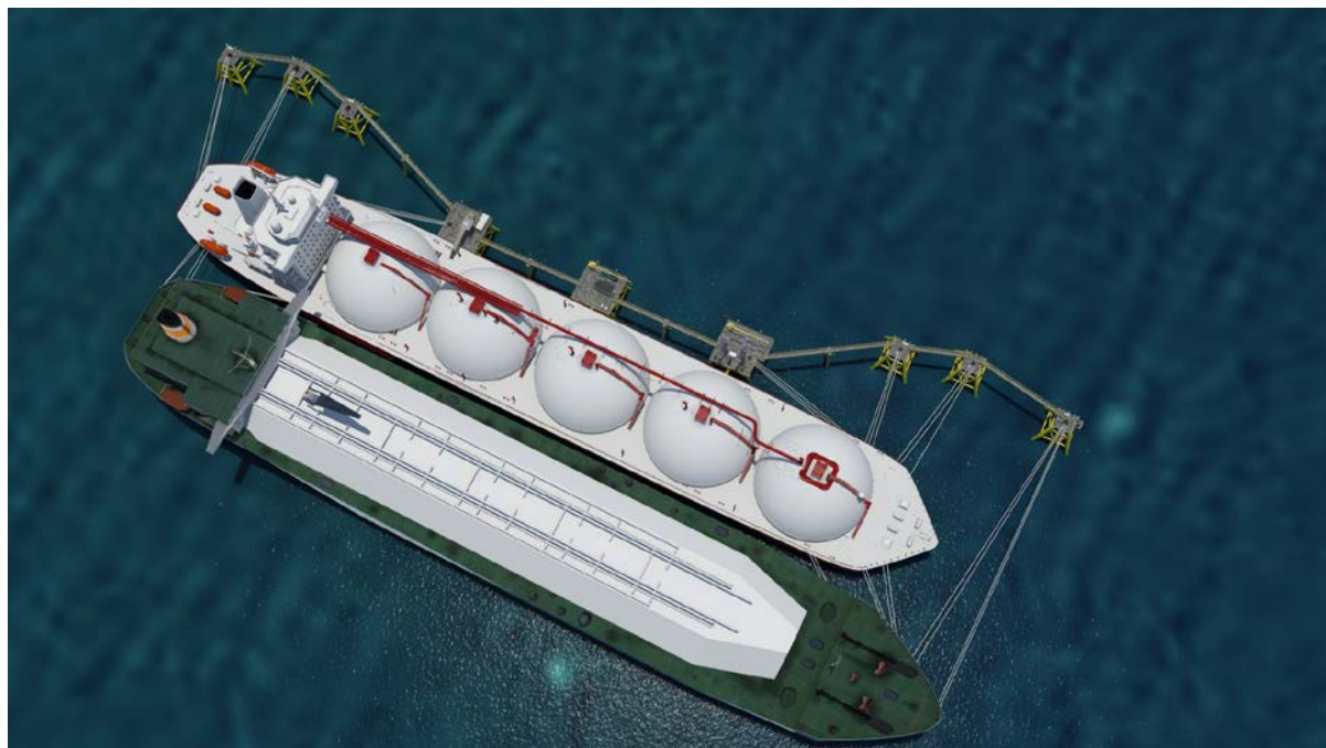
Figure 3. Proposed amendment – larger storage and regasification on FSRU and no terminal for regasification
